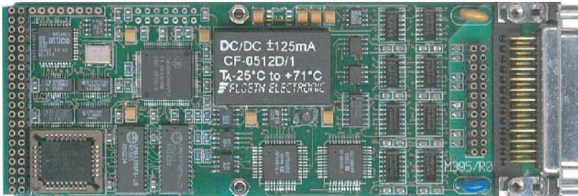
The M395 features 16 analog voltage outputs, integrated on the ANSI certified M-module standard. The digital-to-analog converters have a resolution of 12 or 16-bit.
